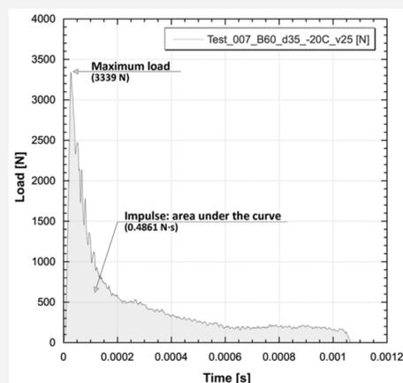
Fig 1 Typical load versus time signal
