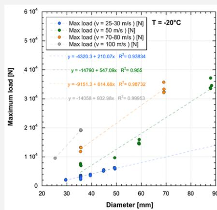
Fig 2 Maximum load for different diameters
