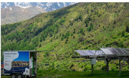
Mobile PV-Lab for I-V-curves, electroluminescence-analysis and high voltage measurements
